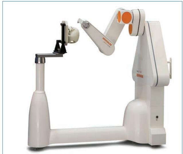
Fig 1. — The neuromate (Renishaw Mayfield, Lyon, France) is a stereotactic system used in various neurosurgical targeting applications. Image courtesy of Renishaw, Inc, Hoffman Estates, IL.
